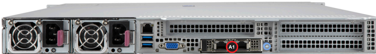
Figure 3-13. AIOM Chassis Slot
